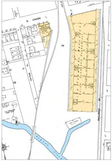
**Figure 2.** The 1913 Sanborn Fire Insurance Map illustrates the property along East Union Street containing the Union Terminal Company Warehouse. It is identified as a fireproof constructed reinforced concrete warehouse built in 1913 divided into 11 bays labelled A through K. *Sanborn Fire Insurance Map from the Duval County Public Library, Special Collections, Volume 2, page 168.*
