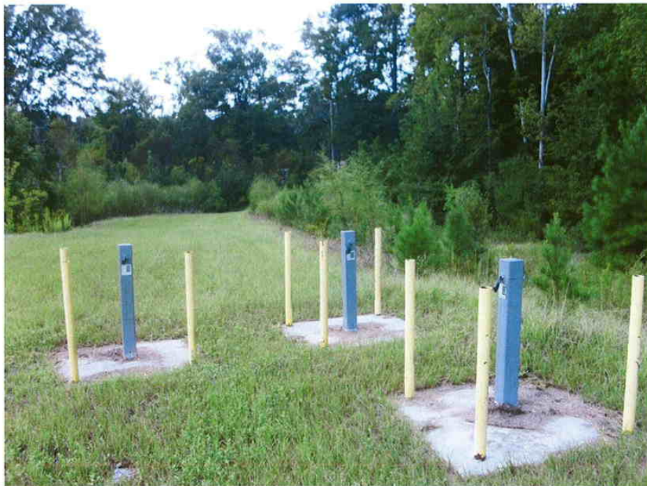
10) View of three groundwater monitor wells associated with the southeastern adjoining property.
