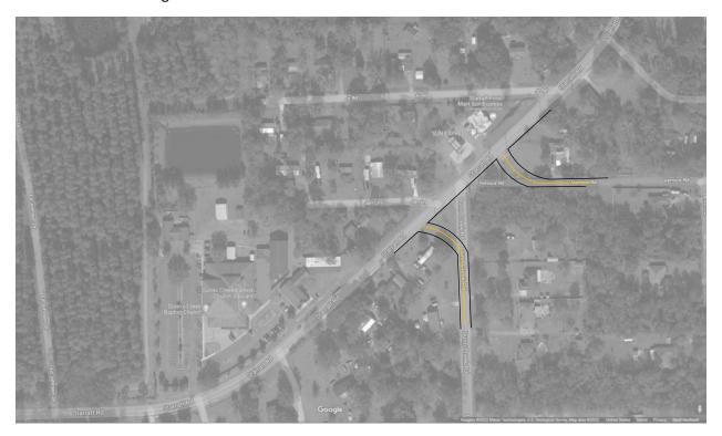
Figure 3 Proposed Reconstruction of Vernice Rd and Dunn Creek Rd
