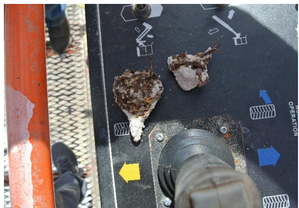
Figure 5. The removed pieces exhibit heavily corroded lath.
